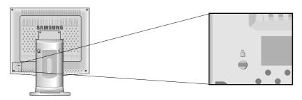
Figure 2. Kensington-type security slot location
